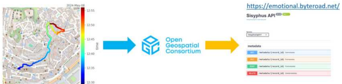
Figure 9. Automated pipeline for synchronizing, georeferencing, and exporting a single or multiple datasets into OGC compliant JSON files to allow direct ingestion to the SDI.
